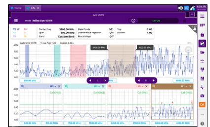
OneAdvisor 800 Cable and Antenna Analysis
