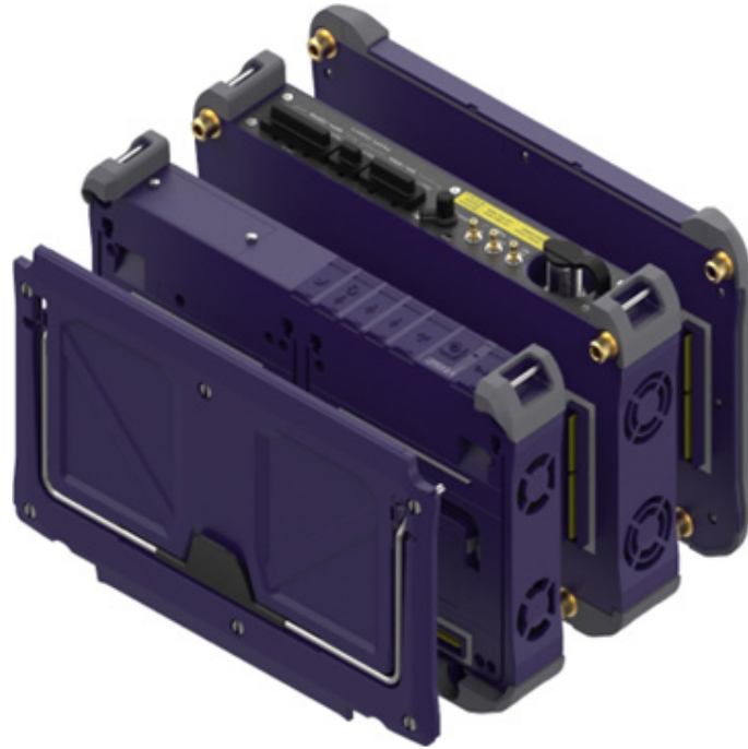
OneAdvisor 800 Expanded View with Full-size Module
